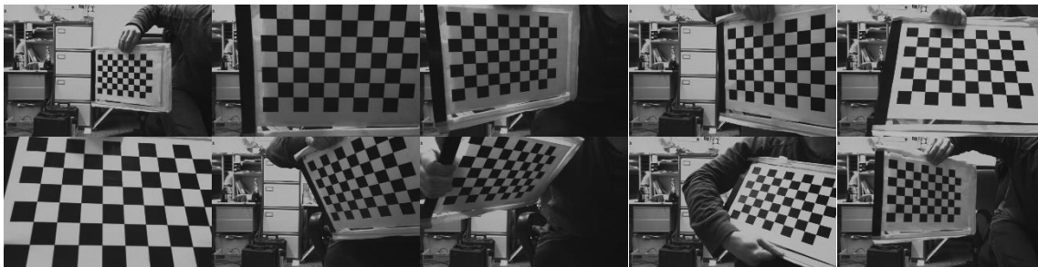
Figure 2 An example set of calibration images, using an A4 target printed on a board.
